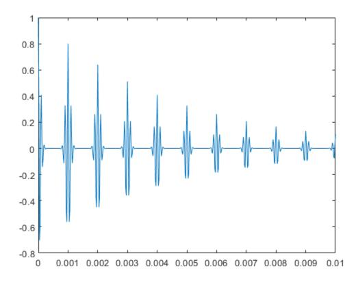
See "Compute Envelope Spectrum of Vibration Signal" for an example that uses the pulstran function to generate vibration data for bearing analysis.
