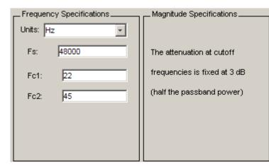
6 After specifying the filter design parameters, click the **Design Filter** button at the bottom of the design panel to compute the filter coefficients. The display updates to show the magnitude response of the designed filter.
